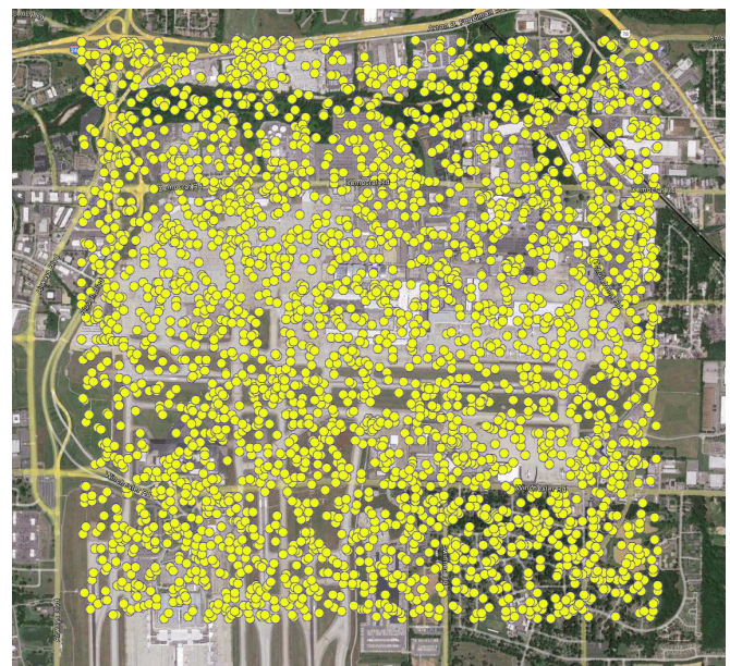
Fig. 5. NLDN-reported cloud-to-ground lightning events at the Memphis FedEx World Hub from 1995 - 2019. Note that all strokes shown have reported peak currents greater than 10 kA.
