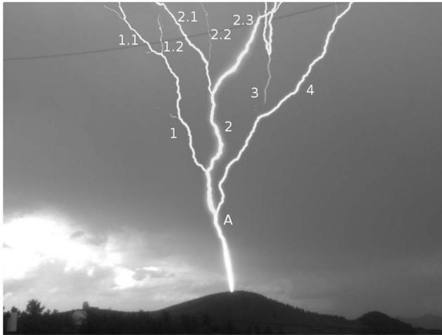
**Figure 1.** Branching of the triggered lightning flash beginning at 20:42:09 UTC on 3 August 2010. Since not all the channels were visible at a single time, the picture is a superposition of images at several times. The luminosity of branch 3 is not graphed in the following figures because it was short lived. The vertical distance from the triggering site to the altitude at the top of the frame is about 1 km.
