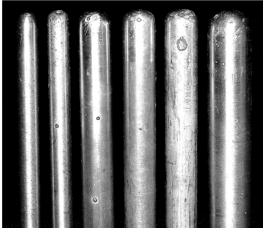
FIG. 9. Photograph of six blunt aluminum rods, each of which has been struck by lightning on South Baldy Peak. The two rods on the left were 12.7 mm ( \frac{1}{2} in.) in diameter, the rod on the right was 25.4 mm (1 in.) in diameter, and the diameters of the other rods were 19 mm ( \frac{3}{4} in.).
